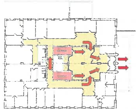
Existing First Floor Egress Path
