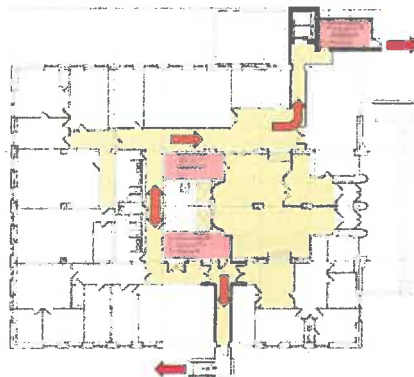
Renovated First Floor Egress Path
