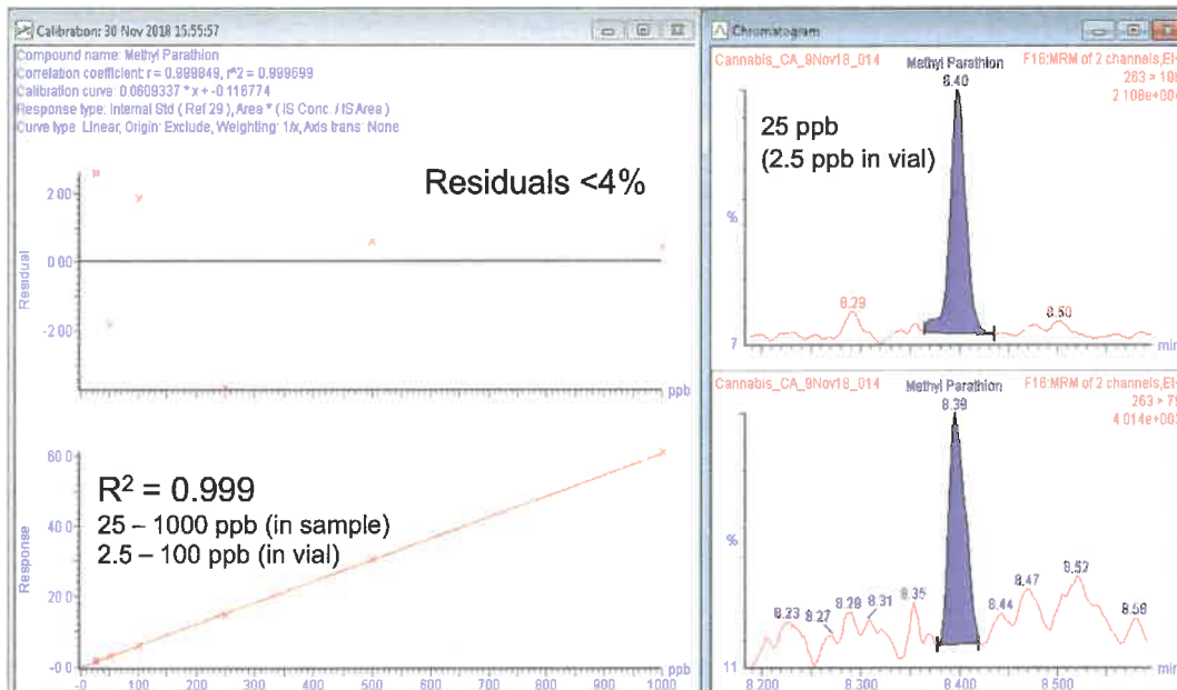
Figure 6. Representative example of a GC-MS/MS quantitation curve for methyl parathion demonstrating a linear range from 0.025 to 1 \mu\text{g/g} (25 to 1000 ppb in sample or 2.5 to 100 ppb in vial concentration).
