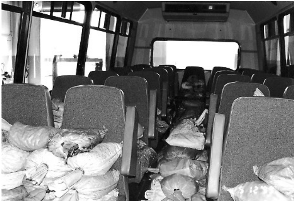
TEST BUS LOADED TO 2.5 TIMES GVL
