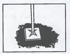
**COMPACT:** Compact with a hand tamper, roller or plate compactor.
