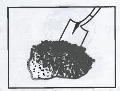
APPLY: Shovel or pour UPM® mix into the hole. Level out 25% higher than the existing pavement to allow for compaction. If patch is deeper than 4", apply and compact in separate 2" layers. Apply only over a solid base.
