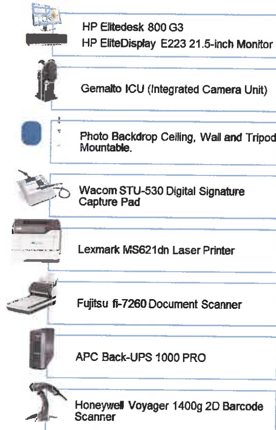
FIGURE 3: ICW WORKSTATION & PERIPHERALS
