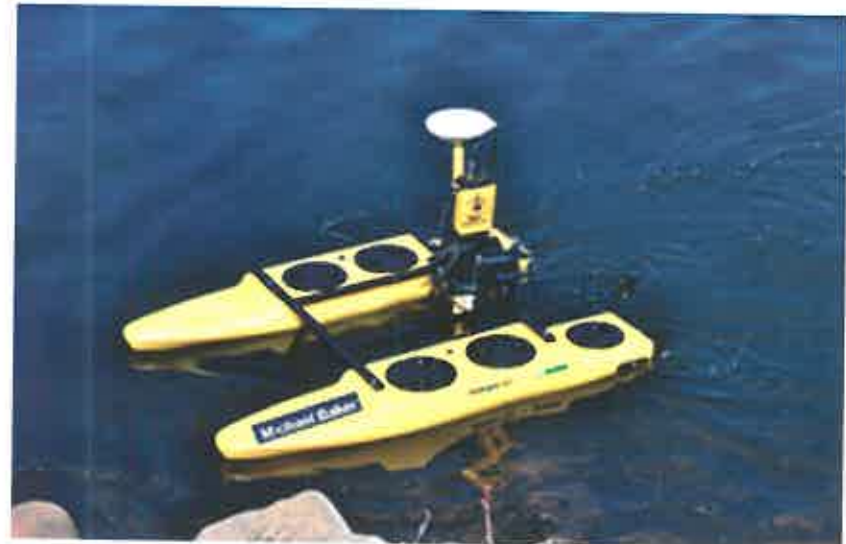
Michael Baker owns a HyDrone bathymetric system and has used it on numerous mine ponds.
