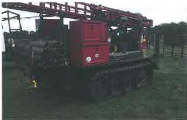
Diedrich D-50 Rubber Track Mounted Drill Rig
