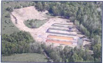
Kimball prepared a site remediation plan for the Laurel Run #2 abandoned mine land site in Indiana County, PA. The project included aerial photography and mapping of the site limits, geotechnical investigations of the existing spoil material, installation of several borehole/monitoring wells above the highwall, design of the acid mine drainage (AMD) remediation technique, and preparation of a construction bid package, as well as periodic site observation during and after construction.
