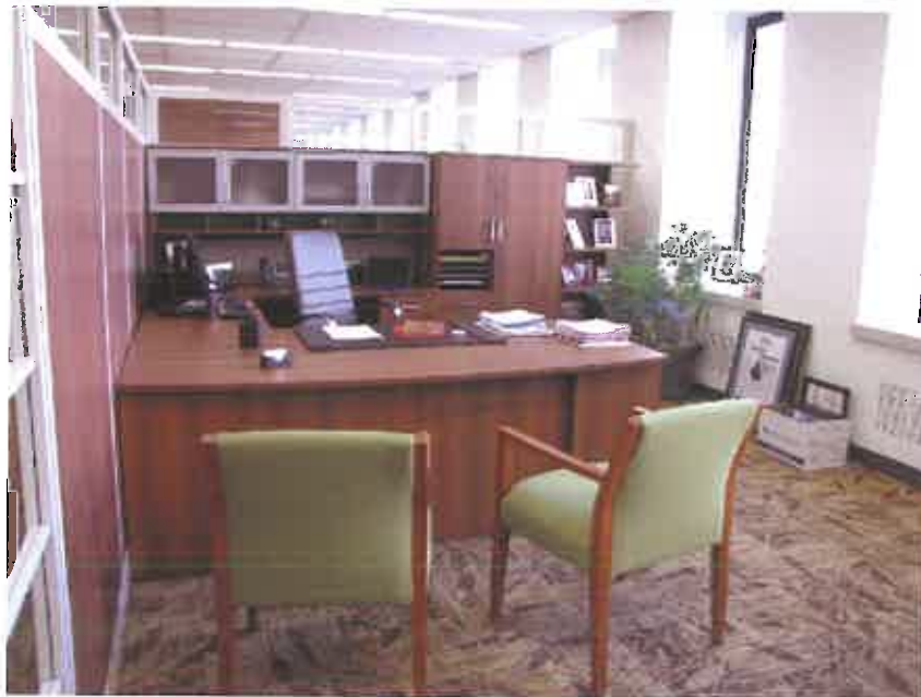
The former Cabinet Secretary's office also includes lower height "walls", and the desk is held away from the return air grilles along the perimeter to allow access.
