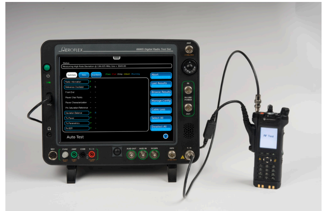
The 8800SX Auto-Test Setup
