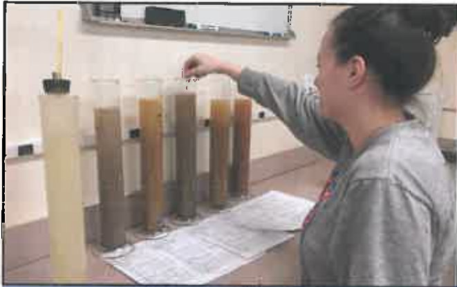
Soil Permeability Testing
