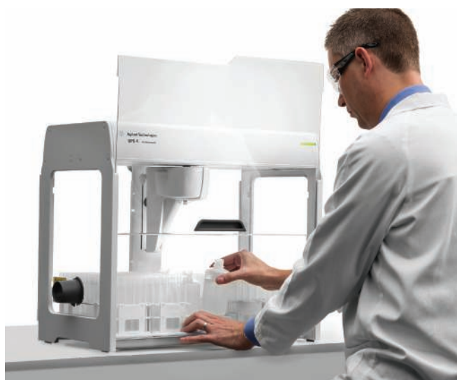
SPS 4 autosampler shown with optional integrated environmental enclosure. Front cover shown in fixed open position for easy access to samples.
