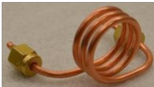
Figure 3. Copper load coil used in most ICP sources.
