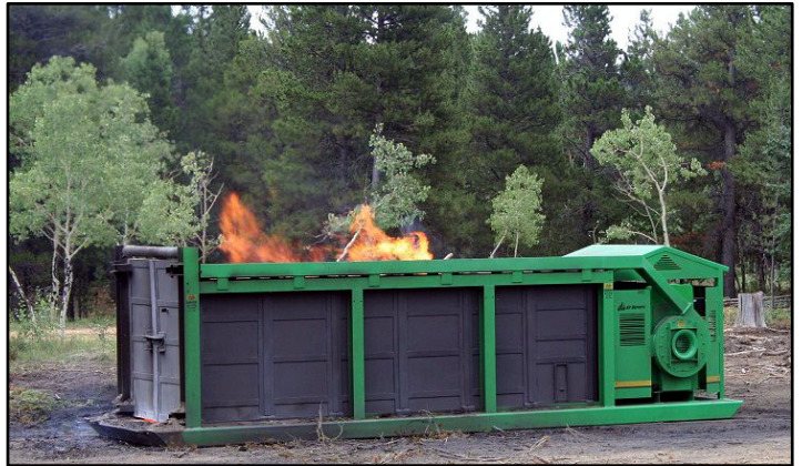
FireBox—No visible PM discharge
