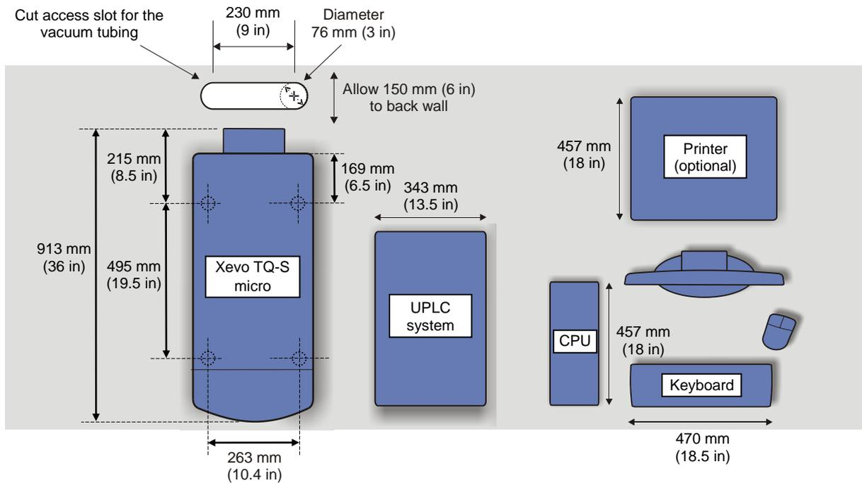
Figure 1 - Plan view, showing space requirements
