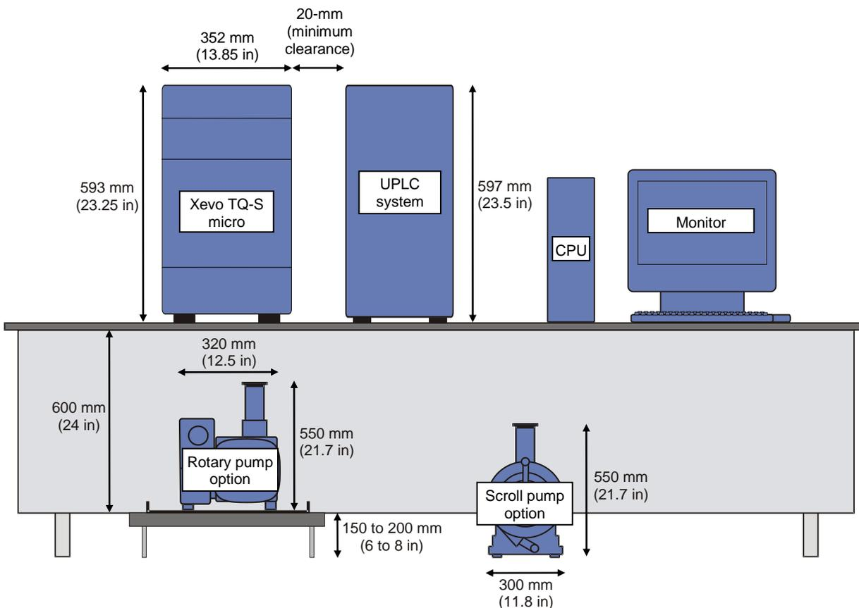
Figure 2 - Front view, showing space requirements
