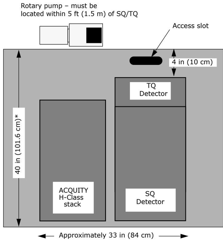
Figure 3 - Space requirements for systems with SQD or TQD mass spectrometers.
