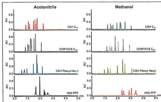
*In developing a method for metoclopramide and its related components, the ACQUITY UPLC H-Class System was configured to automatically screen multiple column and eluent combinations to identify the separation conditions that provided the best chromatographic resolution.*
