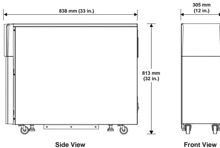
Figure 3 - Approximate maximum dimensions of the UPS
