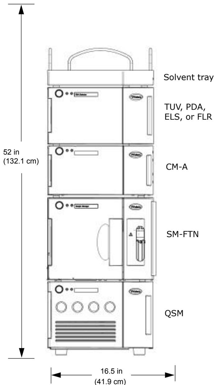
Figure 2 - ACQUITY H-Class System with Column Manager-A
