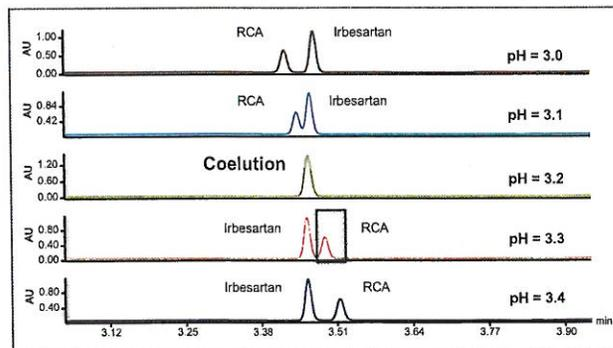
*The USP assay for Irbesartan requires that the eluent be adjusted to pH 3.2, however this results in a co-elution of the API and its related compound. By making automated, online adjustments to the pH in 0.1 increments using Auto•Blend Plus, a more robust set of pH conditions can be found.*
