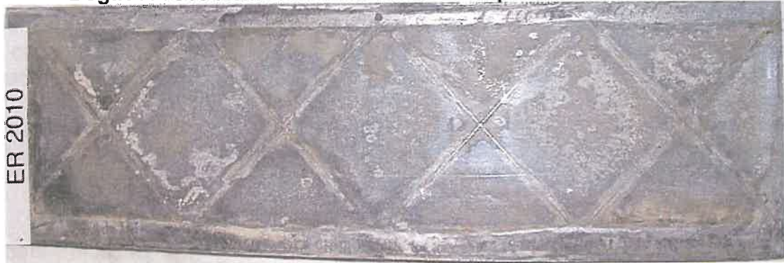
Degacoat 310 Removed After 1500 hrs Exposure to ASTM B117
