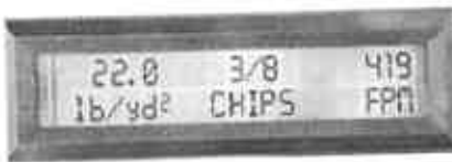
Computer maintains a uniform aggregate application even during changes in road speed. Stores five different application rates.
