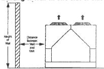
For models AGZ030-100E, maintain a 4 feet minimum from a wall of any height.
