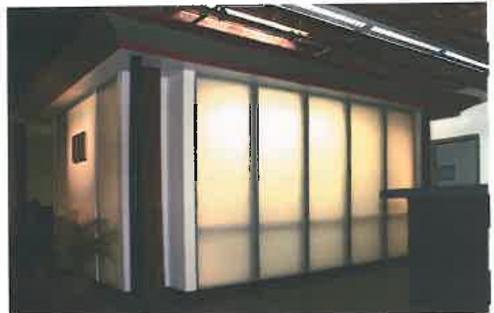
View of our award-winning Charleston Office renovation showing our centrally located conference room "Lantern." This glows all day long through the translucent walls, which are illuminated with natural daylight from a skylight above.
