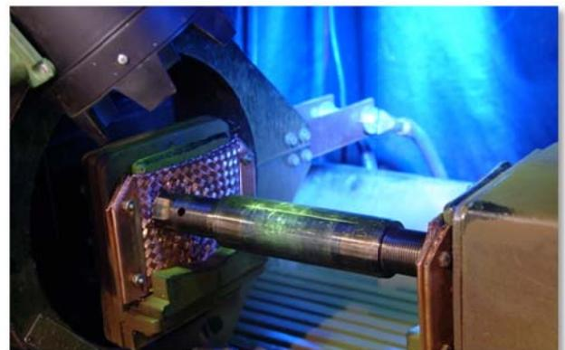
**30,000 lb. & 200,000 lb. Tensile Testers** – Testing externally threaded fasteners for tensile, proof load, and yield strengths; testing internally threaded fasteners for proof loads
