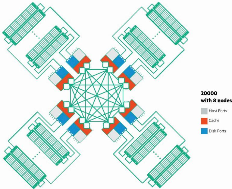
**Figure 2.** Full-mesh backplane of an HPE 3PAR StoreServ 20000 Storage system
