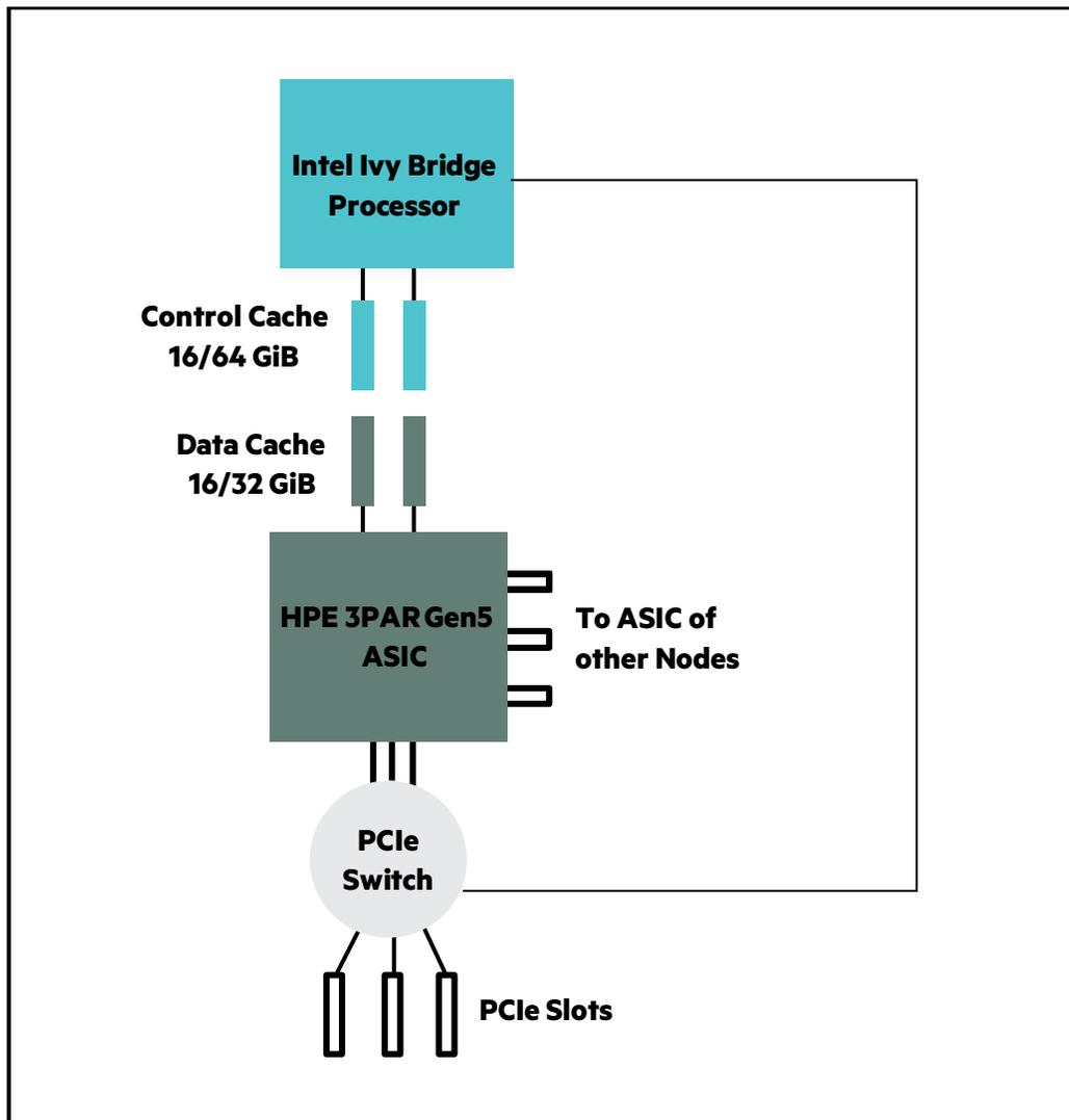
Figure 4. HPE 3PAR StoreServ 8000 Controller Node
