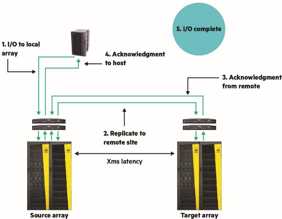
Figure 1. Synchronous mode
