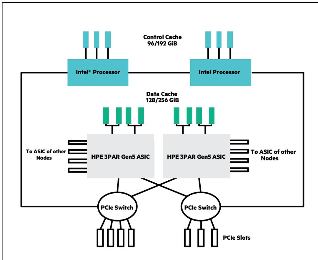
Figure 3. Controller node design of the HPE 3PAR StoreServ 20000 Storage system
