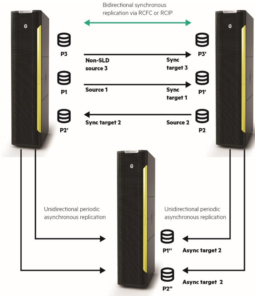
Figure 9. SLD mode: Long-distance replication with zero data loss
