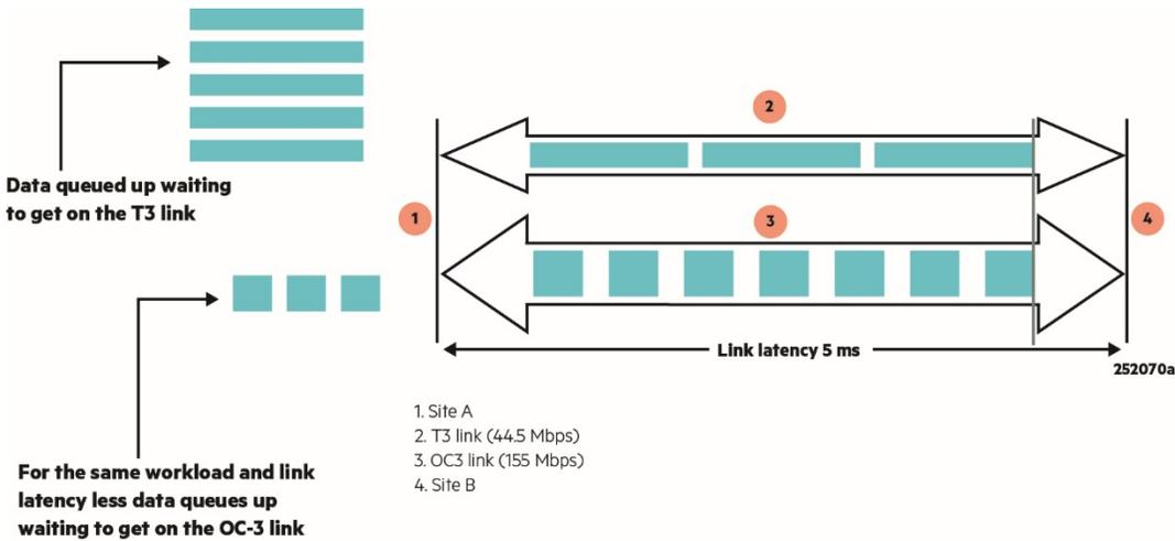
**Figure 4.** Effect of replication link speed on synchronous replication when the data generation rate exceeds the replication link speed
