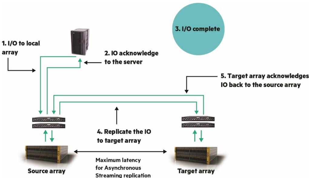
Figure 3. Asynchronous streaming mode
