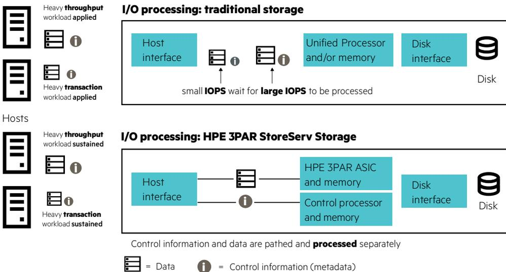
Figure 8. HPE 3PAR StoreServ Storage with mixed-workload support
