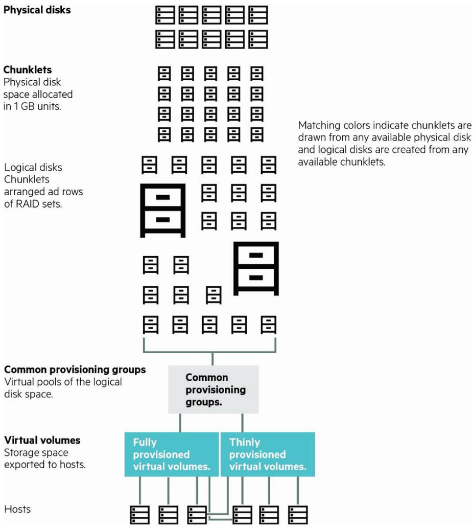
**Figure 1.** HPE 3PAR StoreServ system data layers
