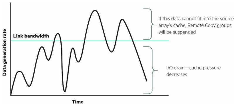
**Figure 5 (a).** Effect of replication link speed on Periodic Asynchronous Remote Copy cache consumption
