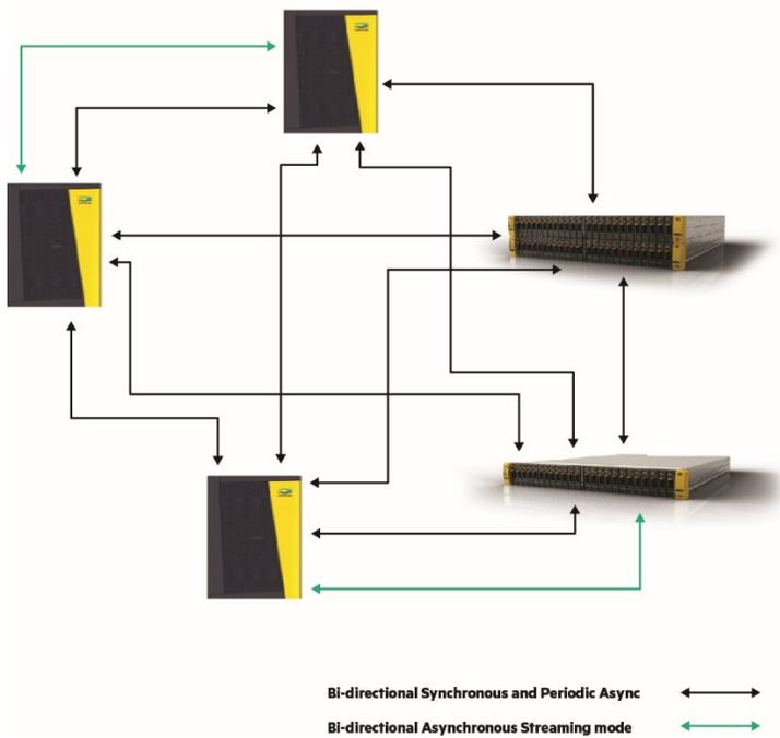
**Figure 8.** Five StoreServ arrays in an any-to-any M-to-N configuration (notice that all relationships can be bidirectional) with asynchronous streaming mode supported between two array pairs
