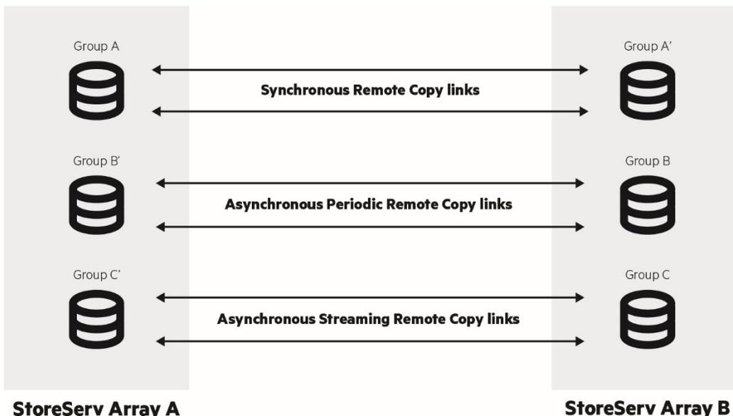
Figure 6. One-to-one bidirectional remote copy
