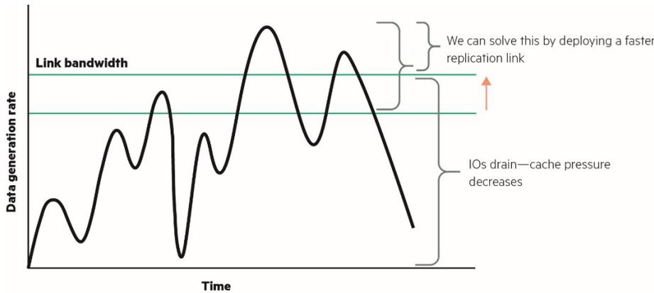
Figure 5 (b). Effect of replication link speed on Periodic Asynchronous Remote Copy cache consumption
