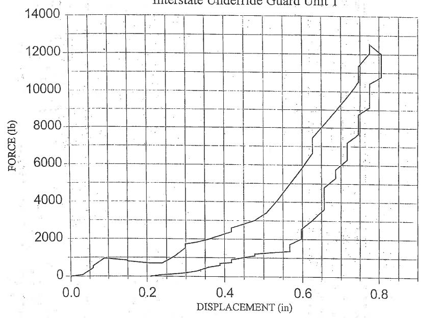
FMVSS 223 Energy Absorption @ P3 Left Interstate Underride Guard Unit 1
