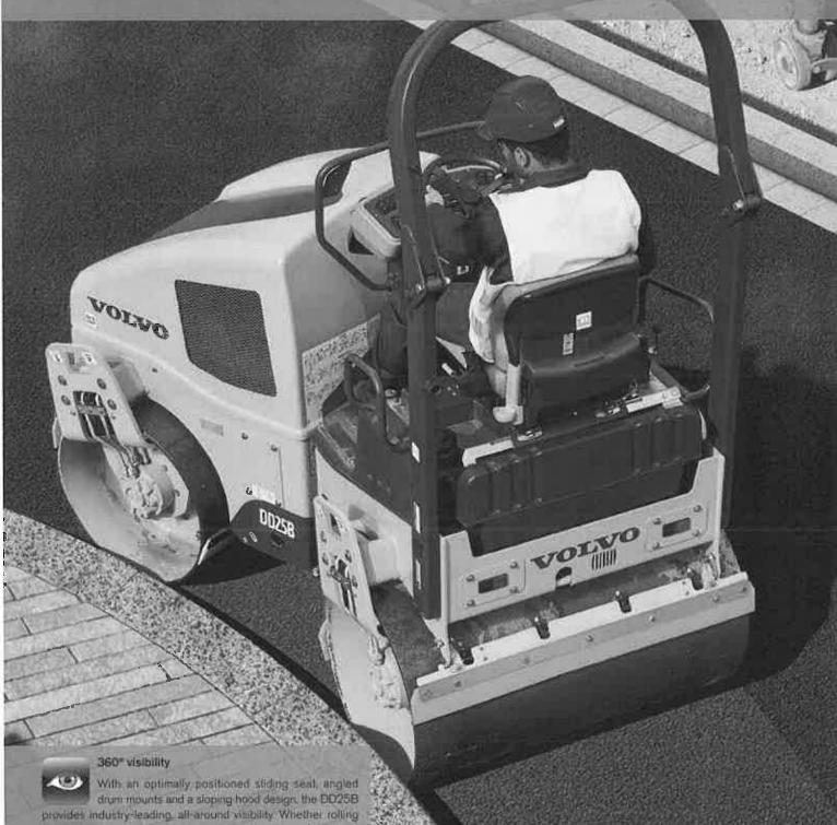
Introducing the DD25B, a highly efficient double drum compactor designed to increase performance and reduce fuel consumption on small scale compaction projects. Featuring the new Volvo D1.7A engine, this machine meets the strict Stage IV/ Tier 4 Final emissions regulations without adding an exhaust after-treatment system. Experience increased machine performance and enhanced productivity with Volvo.
