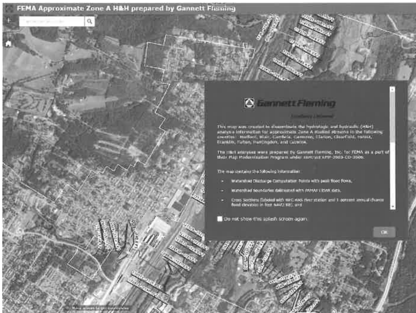
Figure 4-4: Data Dissemination using ArcGIS Online. We developed an ArcGIS Online Web Application to disseminate and view data developed during Map Mod. It includes results from the H&H analyses completed on the Zone A streams in PA.
