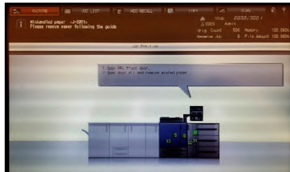
Illustration showing jam locations (above), and a diagram in the centre showing jam location in output module (right).
