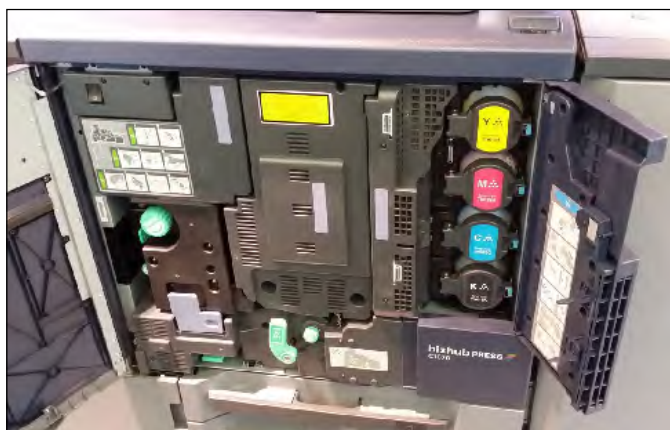
Toner bottles accessed from front of device
