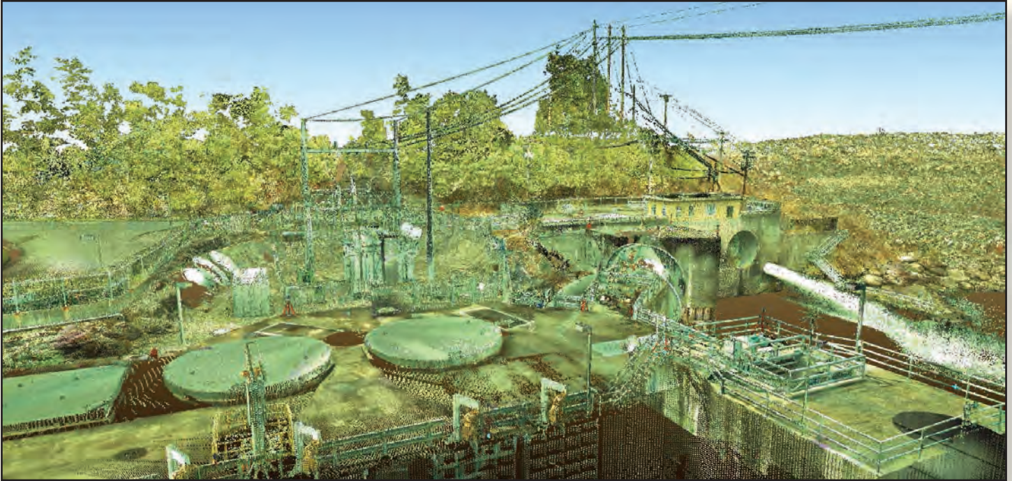
Example of Point Cloud generated from 3D Laser Scanner. (Typically one day of field work for 15 acres or less.)
