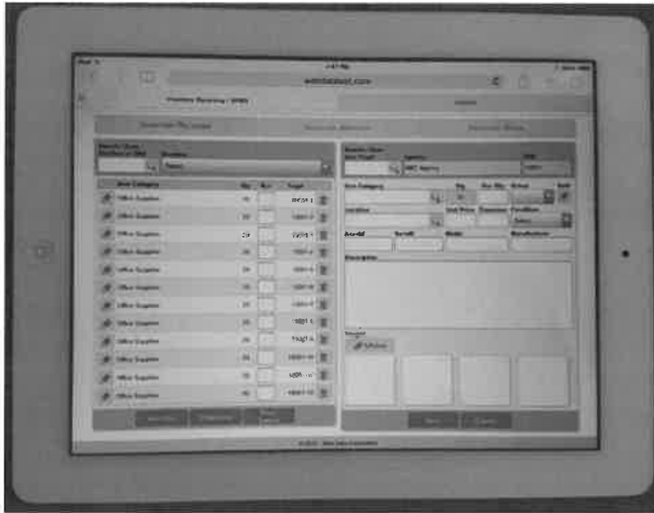
Fig. 40. Tablet screen: State Surplus receiving screen. Receiving of state surplus can be conducted with the scanner device, but also using this screen. Users will tap on a disposal request line item on the left side of the screen and confirm the quantity received; assign a warehouse location; confirm the category; confirm the condition code; optionally add or edit the description using speech recognition; and enter a price and upload images.
