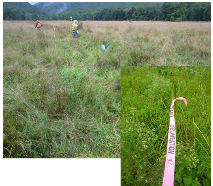
Figure 18: Wetland Delineation and Surveying, WV. Using GPS technology with sub-meter accuracy, we will map wetland and waterway features. If present, wetland boundaries will be marked using biodegradable pink wetland flagging.
