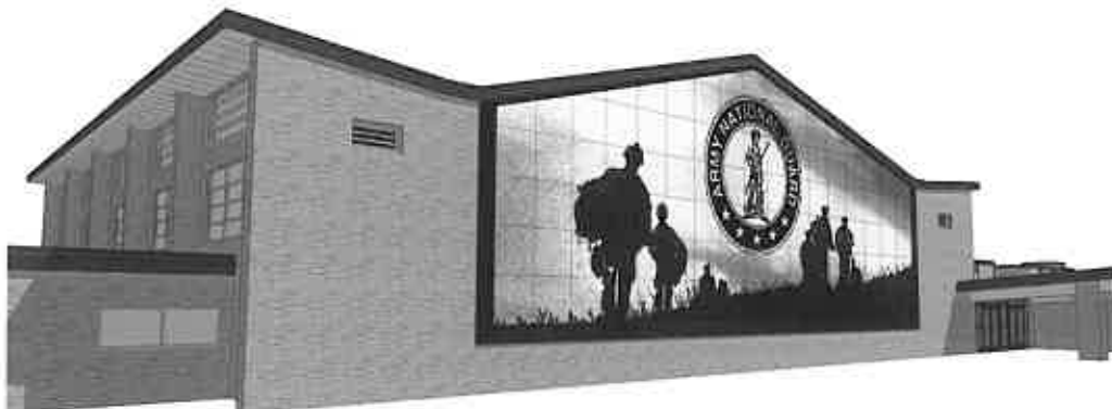
New Perforated Image Metal Panel System Work Package 05 - Alternate A CONCEPT STUDY
