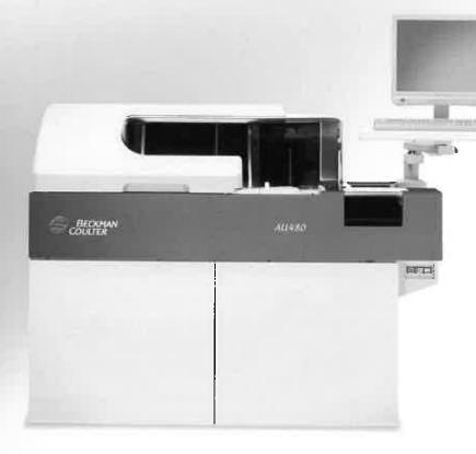
The AU480 is ideal as a primary chemistry analyzer for small- to medium-sized hospitals and laboratories, or as a dedicated specialty chemical or STAT analyzer for larger institutions. With random access throughput of up to 400 photometric tests per hour (up to 800 with electrolytes), 63 on-board parameters and user-definable sample handling options, the AU480 delivers efficiency for all your lab needs.
