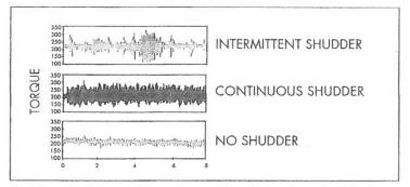
Shudder is disturbing to drivers, who expect comfort and smooth driving. National Multi-Vehicle/MERCON® V ATF reduces transmission shudder, and improves operability and fuel efficiency.
