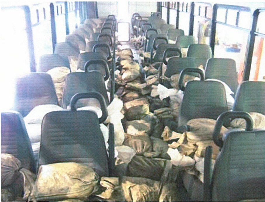
BUS LOADED TO 2.5 TIMES GVL (19,425 LBS)
