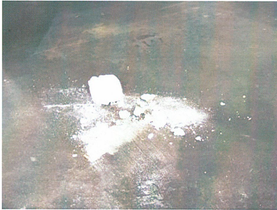
UREA DEPOSIT FOUND AT INLET TO SCR CATALYST
