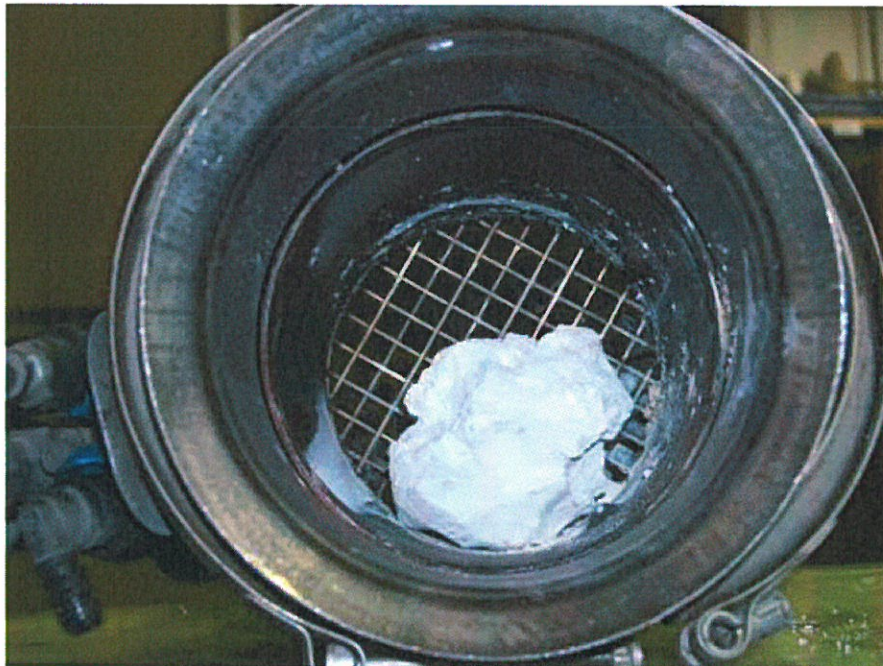
UREA DEPOSIT FOUND AT INLET TO SCR CATALYST
