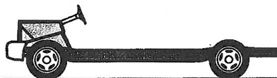
Stripped Chassis: Choice of 138.0", 158.0" or 176.0" wheelbases
