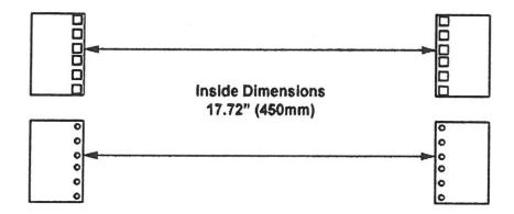
**Front Panel Width:** The only dimension on a 19" rack that actually measures 19" is the width of the front panel of equipment.
