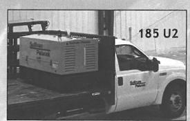
**P2 FlexAir** Machine is built with removable drawbar and running gear so it can easily be mounted on a truck bed or any other utility type vehicle installation.
