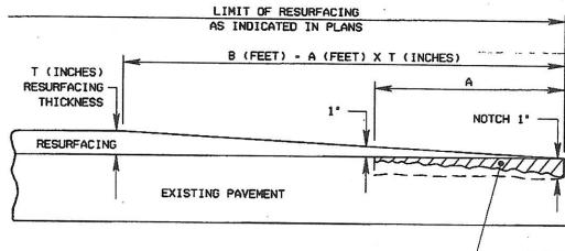
WHEEL RUTS BEYOND THE HEEL-IN NOTCH ARE TO BE FILLED AND TRANSITIONED TO MEET FIELD CONDITIONS.
