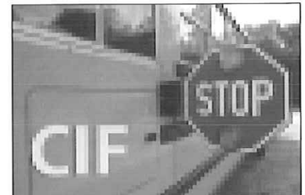
When CIF (352 x 240) is expanded up to 720 x 480 for larger viewing, it produces a poorer quality image.
