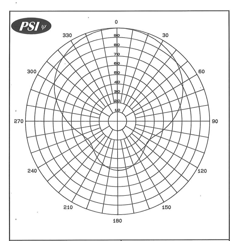
Calculated Relative Field Azimuth Plane Pattern
