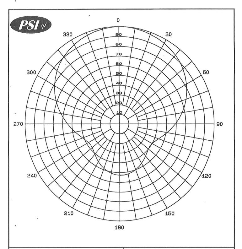
Calculated Relative Field Azimuth Plane Pattern
