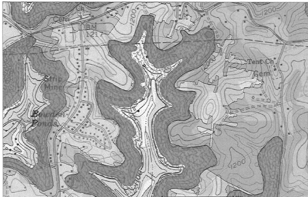
Pittsburgh Coal Mined Out Areas and Structure Contour Map - Ebenezer Run Highwall #9
