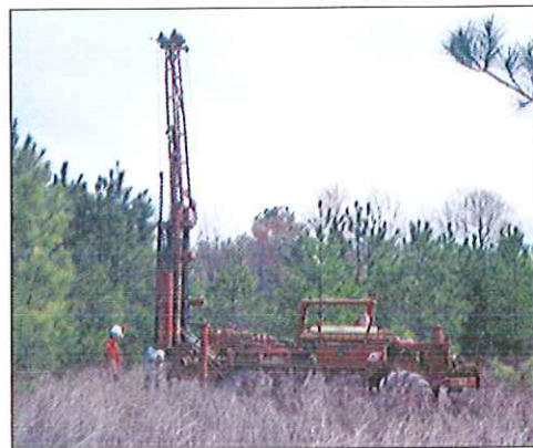
CTL's ATV can drill in rough terrain
