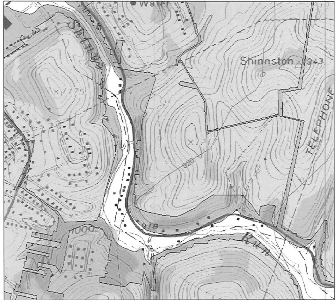
Pittsburgh Coal Seam Mine Out Areas and Structure Contour Map – Shinns Run
