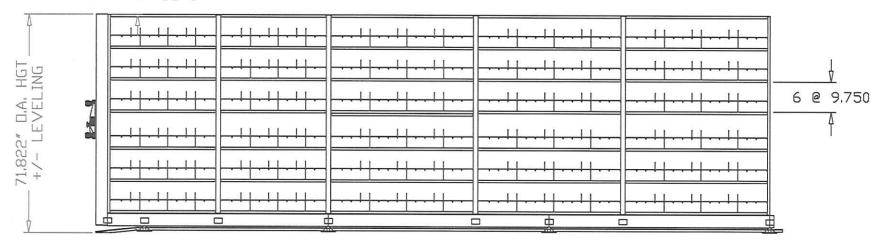
The overall equipment height specified does not include system leveling. A minimum 3" clearance is required between shelving and ceiling/obstructions. This allows for leveling adjustments. A minimum of 18" between shelving equipment and sprinkler heads is required when sprinkler systems are installed.
