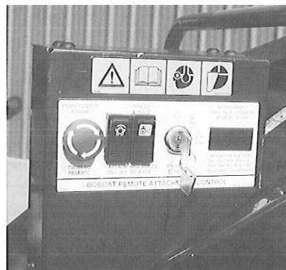
Using the Bobcat Remote Attachment Control*, the operator can start the loader from the ground without entering and exiting the loader. This eliminates the need for a second operator in the loader.
