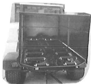
Rear view showing the tubular frame, powder-coated interior as well as exterior components and the industrial processed rubberized rollers.
