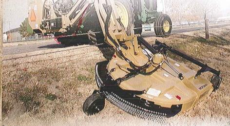
Optional gauge wheel deck allows the cutter to float over undulations without having to constantly monitor terrain conditions.
