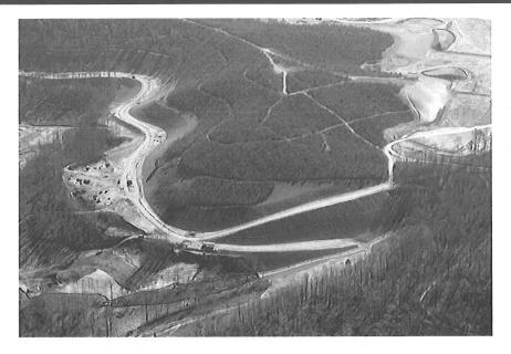
TERRADON has extensive knowledge and experience on all types of AML problem areas. This photo is taken from our Garden Ground Highwalls Project in Fayette County, WV. The photo shows a portion of completed Highwall A on Phase I. The entire project entailed regrading over 14 miles of dangerous highwalls and sealing over 90 portals and will ultimately be utilized by the Boy Scouts of America.
