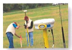
Well trained teams conduct static, real time kinematic (RTK), and real-time differential Global Positioning System (GPS) surveys to deliver accurate mapping and control data for projects. Regardless of the business sector or size of client, our crews provide a wide spectrum of survey services including:
