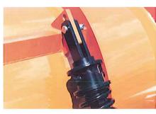
\*ADJUSTABLE TRIP TENSION MOLDBOARD The exclusive, patented, Henderson five-position compression spring settings are easily adjustable to provide variable control of trip force for all snow and ice conditions. (OPTIONAL)
