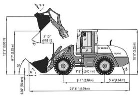
Rate capacity in compliance with ISO 7546: 2.1 yd³ (1.6 m³)
