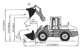
Rate capacity in compliance with ISA 7546:1.6 yd3 (1.25 m3) Max density of material: 2,700 lbs/yd3 (1.6t/m3)
