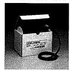
Black rubber tubing has maximum resistance to aging. Withstands repeated sterilization. Durometer hardness: Shore A, 35. Tensile strength: 3500psi. Packaged on 50' reels or In box packs.
