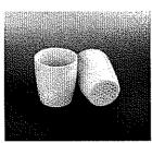
Chemical-porcelain gooch crucibles are used in total suspended solids determinations. Glazed inside and out except outside bottom surface and rim. Perforated bottom. Crucible 89038-046 has two holes for suspending in extraction apparatus. For use in temperatures up to 1150°C (2102°F).
