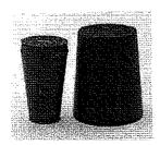
These solid, black stoppers contain a high percentage of pure rubber, weigh less than neoprene, and are low in free sulfur  $\{^1/_2\%\}$ . Composition ensures resiliency and pliability over a long period. Withstand laboratory conditions without hardening.
